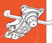
3 Position Back Lock Synchro Tension Adjustment; Turn clockwise to tighten the back tension and counter clockwise to loosen back tension
